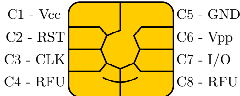
Figure 2.5: Smart card's pin out [Wik14].
