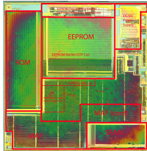
Figure 2.10: Decapsulated smart card chip [IOA12].
