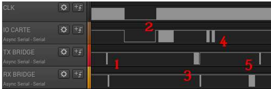
Figure 5.14: Screenshot of the logic analyser output. The computer is sending a cold reset request, the card reboots, then the computer sends a test case to be applied to the card. The card answers and the response is sent back to the computer through the bridge.
