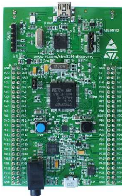
Figure 5.2: Picture of the STM32F407 Discovery board provided by STMicroelectronics taken from its user manual[17]. The main chip in the middle is the STM32F407 microcontroller, which is surrounded by all the necessary equipment to make it run while easing programming and debugging.
